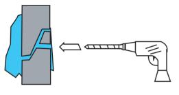
Drill 5/8" diameter hole to intersect leak path
