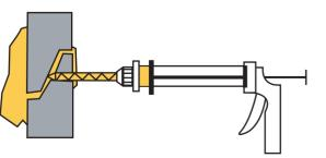
Pump gun vigorously to expel grout to refusal or seal. If grout is washing out either pump slower or stop pumping and watch grout until it reacts halfway down A (mixer) then quickly give a pump to expel and repeat.
