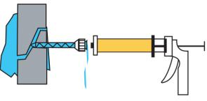
Prepare gun by pulling back plungers on E (dual caulk gun) insert D (tubes) while holding vertical, remove C from threaded end of tubes Quickly align threads on D (tubes)
