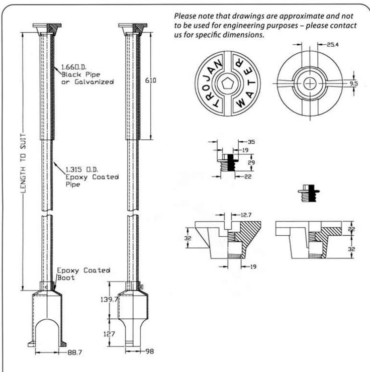
Material: 1.66 D.D. Upper section 1.315 D.D. Casing-ASTM A-500 Type 1 HRR Steel Cast Iron Cap and Boot- ASTM A-48 Class 20 Grey Iron 1.315 D.D. Casing Epoxy Coated Brass Pentagon Plug - CDA 60-40 Yellow Brass
