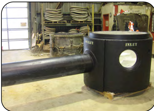
HDPE cast into barrel - watertight.
