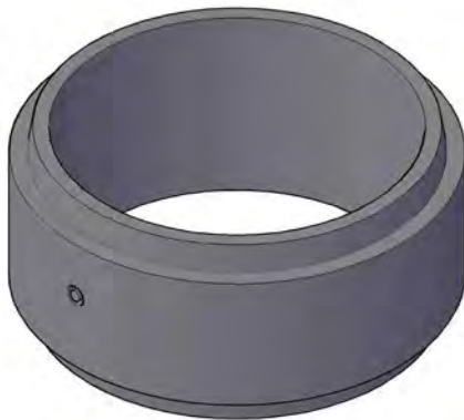
ISOMETRIC VIEW OF 1220 Ø BARREL SPIGOT / SPIGOT ADAPTOR
