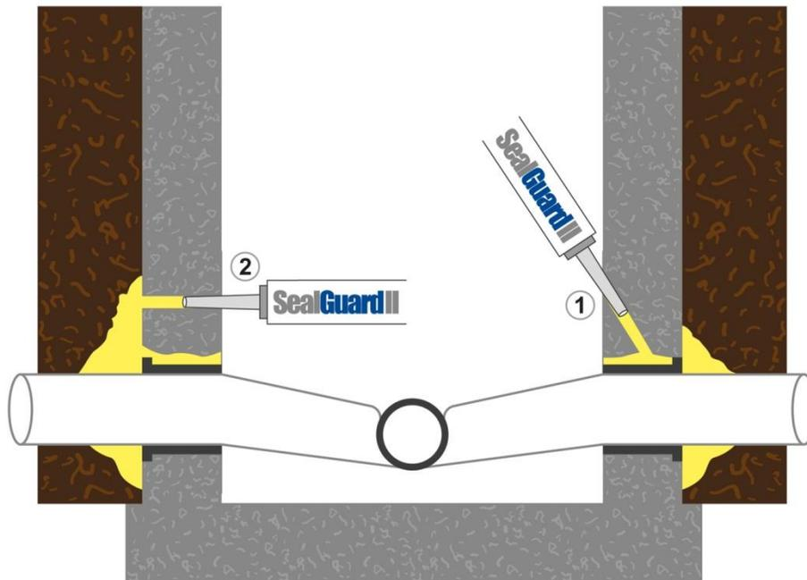
While this drawing is of a manole, it illustrates the principal of drilling through the substrate on the left, intersecting the leak path on the right.
