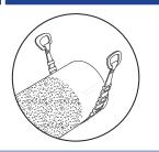
Prepare pipe end by de-scaling if required. Clean the pipe as required with water. Make sure that the pipe is clean from debris and defects that interfere with HYMAX GRIP's proper seal.
