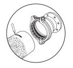
Mark pipe end to a minimum required stab depth as indicated on the product label. These marks indicate the required stab depth of the pipe on the HYMAX GRIP Open Bore Flange Adaptor.
