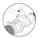
Connect the HYMAX GRIP Open Bore Flange Adaptor to the flange and tighten bolts.
