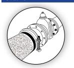
Position the HYMAX2 Flange Adaptor. Once the gasket is properly sized, position the HYMAX2 Flange Adaptor over the pipe end covering the marks on the pipe (step 4). For uncoated ductile iron, grey cast iron and asbestos cement pipe surfaces, appropriate gasket lubricant is required on both the inside surface of the gasket and the outer pipe surfaces.
