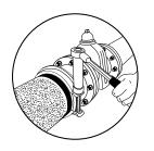
Tightening the end rings. Tighten the Flange Adaptor's bolts using a 3/4" socket wrench for 2"-3" couplings, a 7/8" socket wrench for 4"-12" couplings. When you finish, re-check the torque again.
