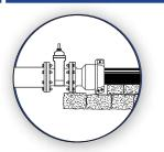
Unpack the HYMAX2 Flange Adaptor. Carefully remove it from the packaging. Inspect the HYMAX2 Flange Adaptor for shipping damage and verify that there are no missing parts.
