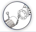
Prepare the pipe end. Clean and de-scale pipe end. Remove any debris or build up on the pipe end and clean the outer pipe surface with soapy water. Clean pipe end to a distance that is equal to the length of the center ring. Make sure there is no corrosion on the outer pipe end that could affect the gasket seal. Again, clean pipe end with water.
