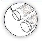
Measure the pipe's outer diameter and make sure the adaptor's size will fit properly.
