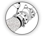
Assemble the flange joint using flange bolts. Make sure you use a flat gasket between the flanges (not provided).
