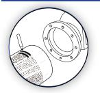
Make 2 markings on the pipe - one for the closed position of the gasket and one for the open (flip) position. The mark for minimum stab depth which is closer to the product is at a distance of 2.25" from the edge, the mark further away at 3.25", which is for the open gasket position.
