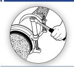
Tighten the end rings. Tighten the coupling bolts to the right torque shown on the product's label. When you finish, re-check the torque again.
