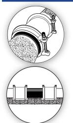
Position the coupling for installation. If possible place the couplings on the replacement pipe with top-facing bolts and lower the pipe and couplings into the ditch. Slide the couplings outward so that it covers the marks made in step 3. Make sure that the pipes are not touching inside the body of the HYMAX. There must be space between the pipes in order for continuous dynamic deflection to take place.
