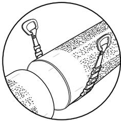
Prepare the pipe ends. Clean and de-scale each pipe end. Remove any debris or build up on the pipe ends. Clean the outer pipe surface with water. Clean each pipe end to a length of the coupling body.
