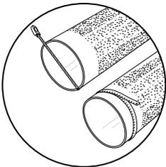
Measure the pipe's outer diameter and make sure the coupling being used has the proper OD range. Always use an OD tape to ensure that you are using the proper size coupling
