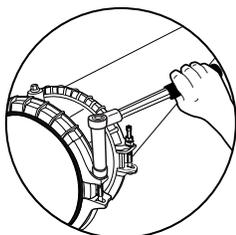
Tightening the end rings. Tighten the coupling bolts using a 15/16" socket wrench for 14"-24" couplings, and a 1.5" socket wrench for 26"-60" couplings. Tighten the bolts evenly on each end ring in an alternating pattern to the torque mentioned on the label. Cross-tightening ensures that the gasket is evenly seated. When you finish, re-check the torque again.
