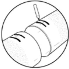
Mark the pipe ends according to the following stab depths, with two lines on each pipe end (minimum and maximum):
