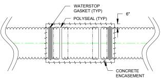
outside edge of the concrete collar. Typically, approximately 6" (0.15m) is excavated beneath the pipe to allow for proper application of the *Polyseal* coupler and concrete encasement. If the pipe itself is damaged, the damaged area shall be removed and a replacement pipe section spliced in prior to pouring the collar. This repair option may be employed for either dual wall or triple wall sanitary pipe.
