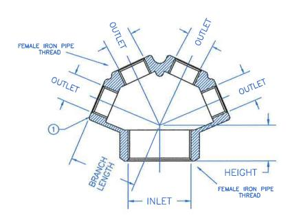
PARTS AND MATERIAL: 1. BODY: CAST BRASS, ALLOY C89833
